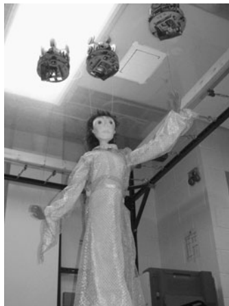
Figure 27.3 Three robotic controllers operate a wooden marionette suspended from a plastic ceiling that covers a stage at the McCormick School for Engineering at Northwestern University: the robots each control two puppet strings and collaborate with each other to generate marionette motion; Evanston, Illinois (January 2011). Photo courtesy of the authors
