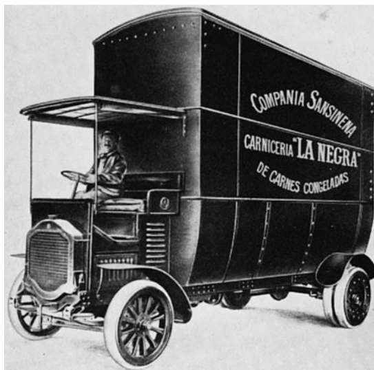
Figure 12.6 Insulated motor van. From J.T. Critchell and J. Raymond, History of the Frozen Meat Trade (London: Constable and Company, 1912)
