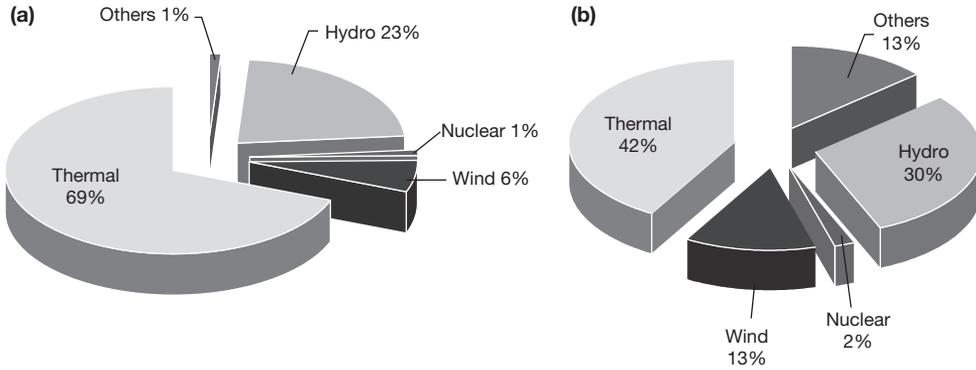
Figure 16.5 Structure of China's generation capacity, 2013. (a) Total installed capacity. (b) Newly installed capacity
