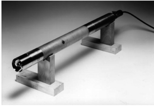
Figure 3.8 Cambridge self-boring pressuremeter (courtesy of Cambridge Insitu)
