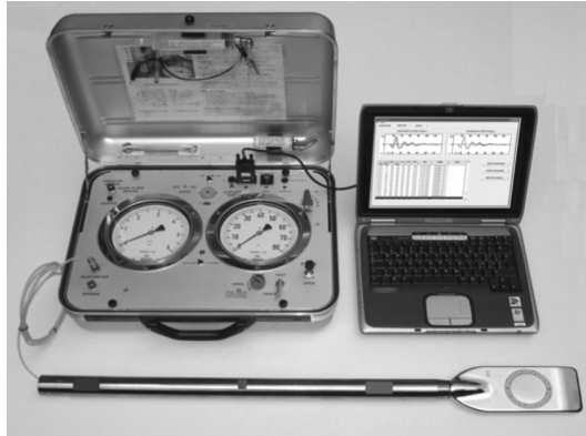
Figure 3.12 The seismic dilatometer (courtesy of Marchetti)
